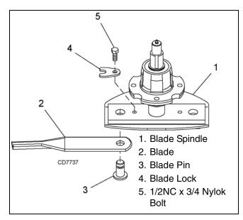
Figure 12. Blade Removal
